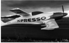
modifications include an extra aux tank which is 11 gallons under the rear wing, a new style gear, larger rudder, and redesigned tail.
